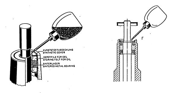
When replacing the plastic cap, one has to make shure it is pushed home fully to its stop, as it may otherwise touch the cover plate.
